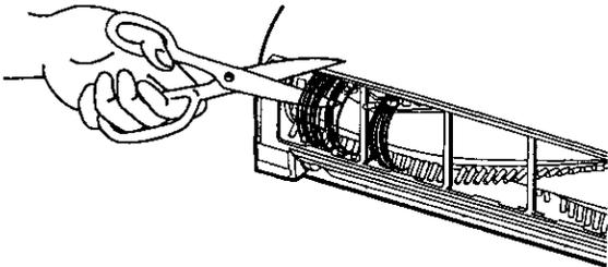
To clean agitator turn vacuum cleaner over, cut off any carpet pile and lint entangled around agitator with a pair of scissors as shown.
